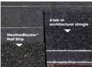
3-Tab & Laminate Shingles: When up to an 8.5"- (216 mm) width starter strip meets the need, simply tear the starter shingle in half along the perforations
